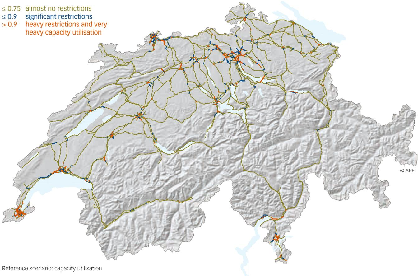
Reference scenario: capacity utilisation (vehicles/capacity) of the high-capacity and major road network, 2040.
